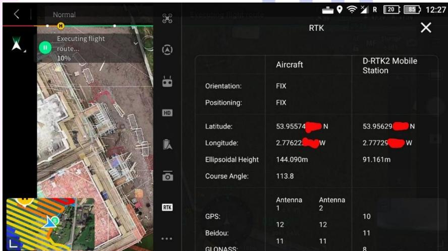
For this flight, the DRTK3 was again used for base corrections, but I manually entered the coordinates of the known point created earlier, as the DRTK3 location.
