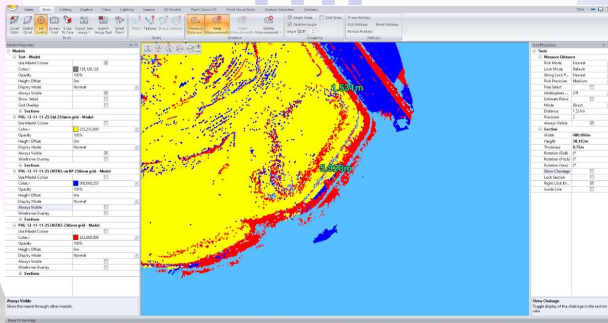
Vertical alignment also varied. Depending on the location, height differences ranged from a few millimetres to a few metres. Again, Flight 3 (blue) generally performed better than Flight 2 (red), though still not perfectly.
